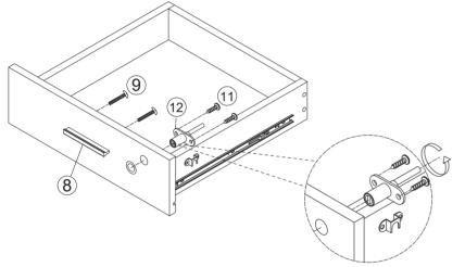
When installing the lock cylinder, please keep the column of the lock cylinder can only be rotated on the right side
