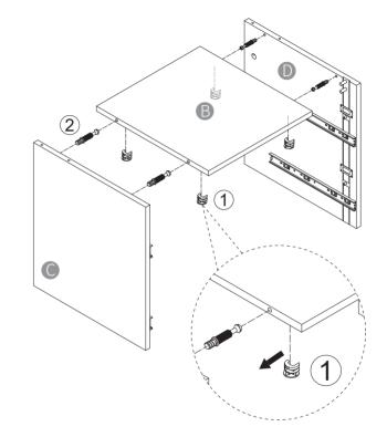
Please point the arrow to screws holes when installing the eccentric gear, and tighten it clockwise to fix the board after installing the board.
