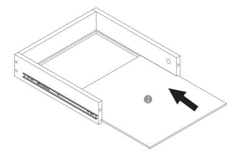
Please point the arrow to screws holes when installing the eccentric gear, and tighten it clockwise to fix the board after installing the board.
