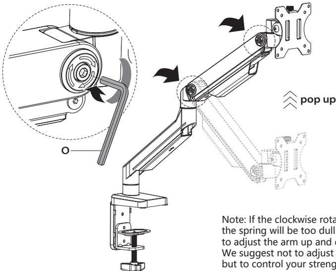
Note: If the clockwise rotation is too tight, the spring will be too dull and it is difficult to adjust the arm up and down. We suggest not to adjust it to be too tight, but to control your strength.
