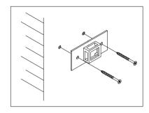
Install the accessories onto the wall as shown in the diagram
