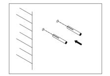
Mark on the wall according to the height and width of the top board A, and drill holes at the marked position with an electric drill, put fittings into the holes
